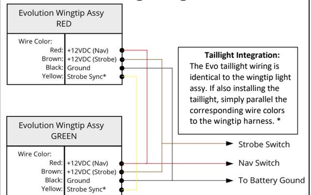
\*To synchronize strobe flash between both wings and/or tail (not required), yellow wire from each assy must be spliced together to each other. DO NOT attach the yellow wire to power or ground.
